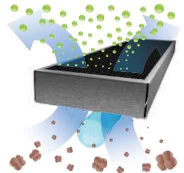
Odors, bacteria, viruses and other complex airborne contamination are drawn through the activated carbon modules
